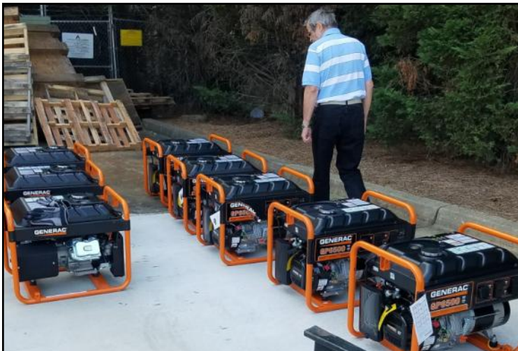
Generators were fueled, run dry, and had their oil drained to be ready for shipment
