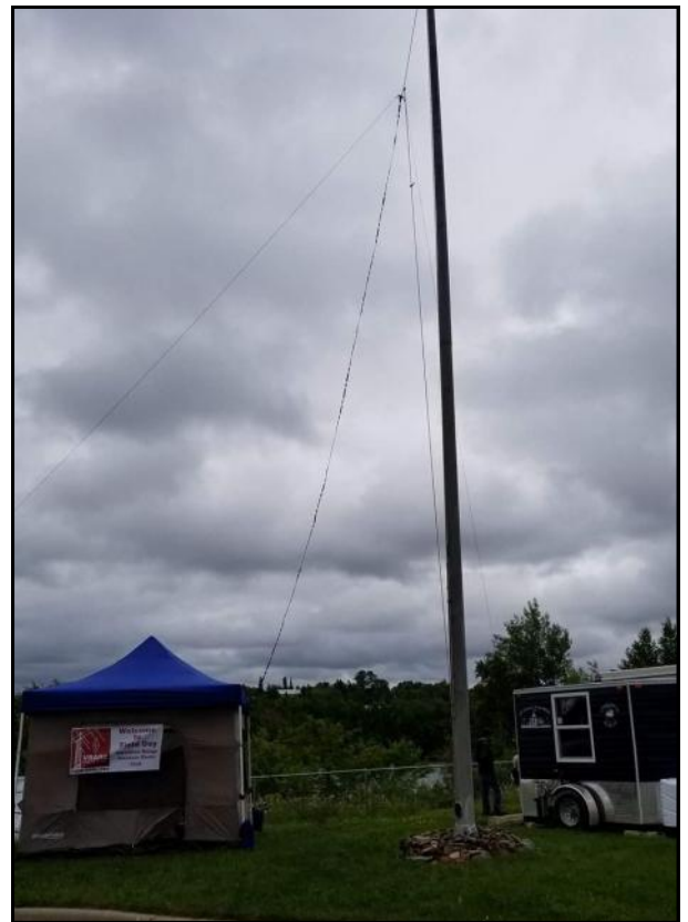
Dipole from the Flagpole; Antenna for the first Vermillion Range Amateur Radio Club Field Day at Pioneer Mine in Ely MN.
