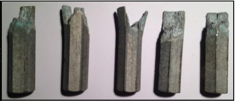
Most of the standoffs that held the 40M linear loading wire had deteriorated pretty badly over 10 years
