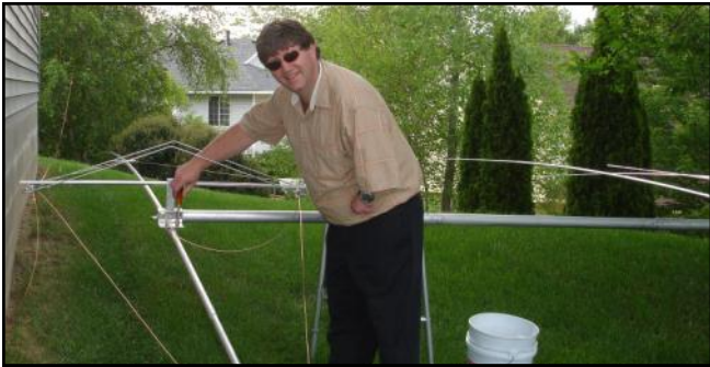
One of the original 40 meter elements using the linear loading wire. Pictured is KTØR (SK)
