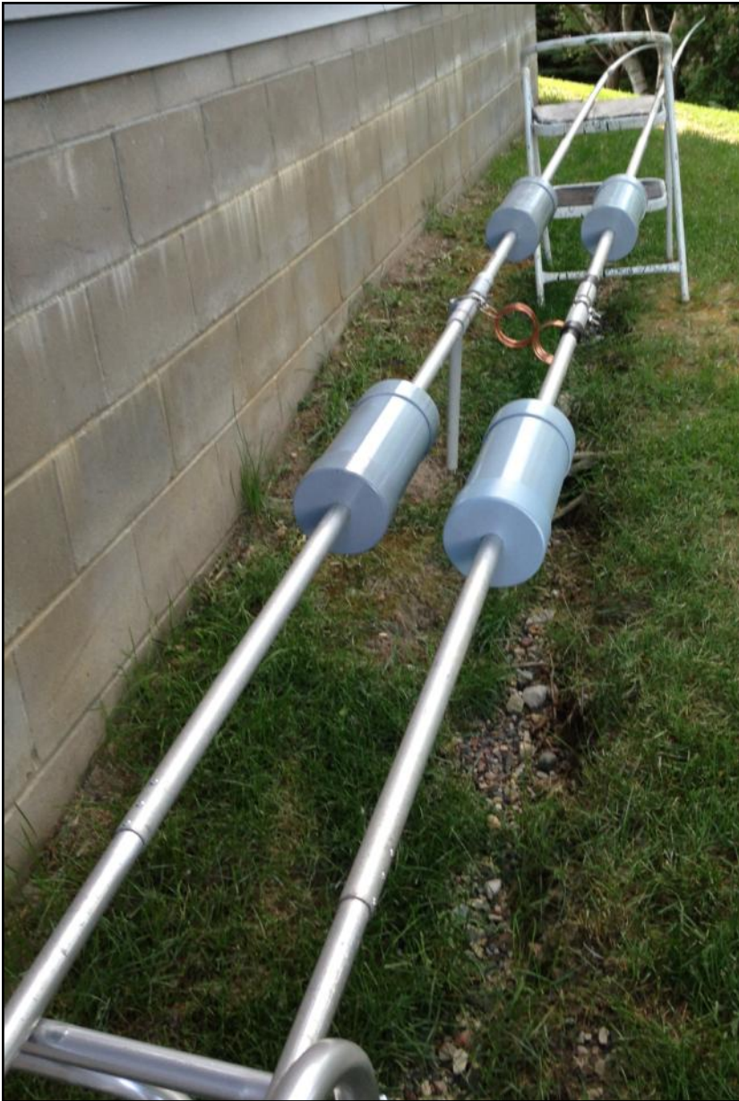
The completed 40 meter elements ready to raise and install on the boom
